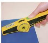
涂层厚度测定 Coating thickness measurement
